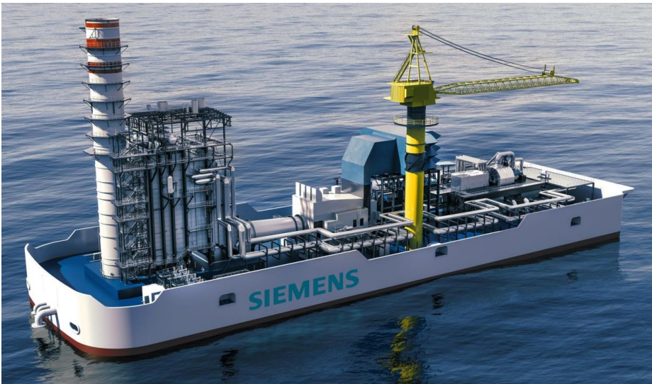
Figure 9: Typical 700 MW CCGT Floating Power Barge.
