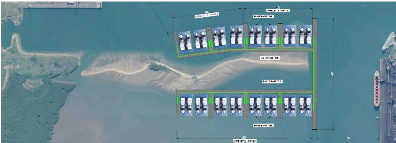
Figure 54: Layout 2 for the NIFPP within the Port of Richards Bay, essentially enclosing the Sand-spit
