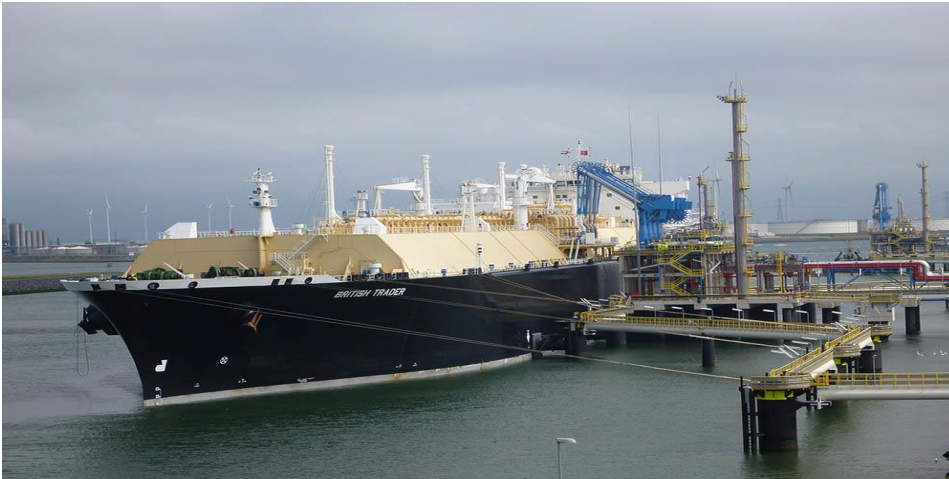
Figure 5: LNG FSU permanently moored/ berthed to the LNG Terminal’s docking/ mooring station (offloading platform).
